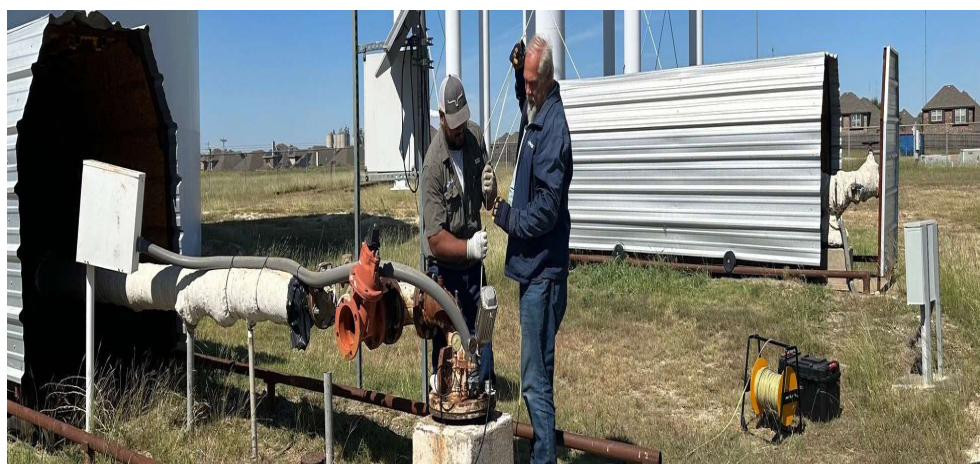
Field Technicians, Jose Sarmiento and Rusty Zent, collecting water level data by e-lining a monitor well.
